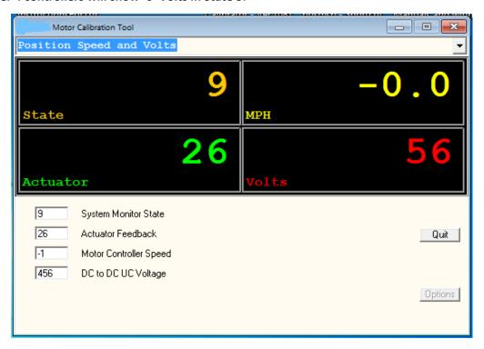
By cycling the driver switch on and off, the state and actuator movement can be determined for proper operation.
