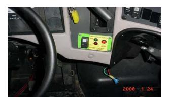
**Normal Running** – With the ignition ON, engine running, hybrid rocker switch ON and vehicle stopped – the Green light should be ON and the red light should be OFF.
