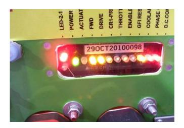
LED-2-1: Upper light flashes Red indicating initialization of controller & Driver switch off. Lower light (Green) is on when Driver switch is on and system is ready.
