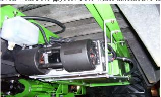
v. **IF NO** to c.i and c.ii – unplug connector on cooling module and reinsert plug firmly. **IF Not OK**, check power at J205, pins 1 & 2 (12 vdc) to 7 & 8 (ground) **IF Not OK**, Go To section a.iii (40 amp fuses).
